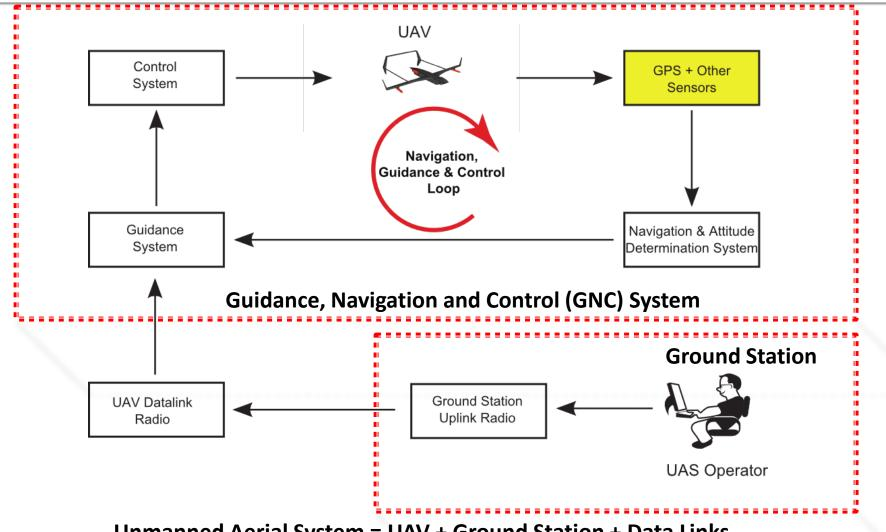
Unmanned Aerial System = UAV + Ground Station + Data Links
